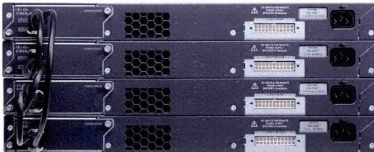
Figure 5. Cisco FlexStack-Plus switch stack
